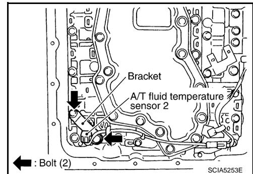
6. Remove bracket from A/T fluid temperature sensor 2.
