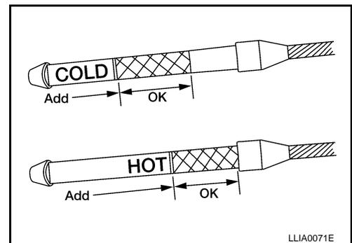
8. Install the A/T fluid level gauge in the A/T fluid charging pipe and install the A/T fluid level gauge bolt.
