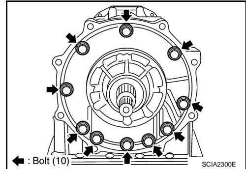
7. Remove the oil pump assembly evenly from the transmission case using Tools.
