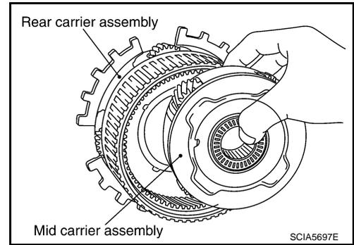
18. Remove needle bearing (front side) from mid carrier assembly.
