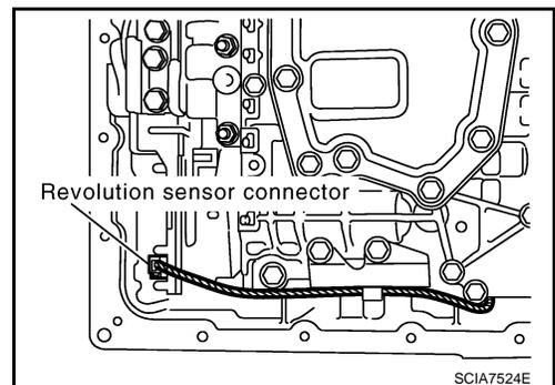
13. Securely fasten revolution sensor harness with terminal clip.
