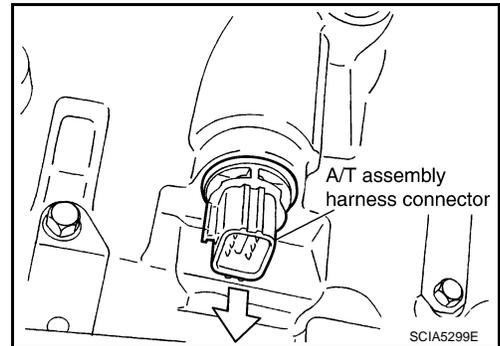
15. Install snap ring to A/T assembly harness connector.
