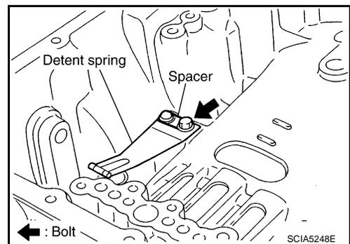
3. Install manual shaft to transmission case.
