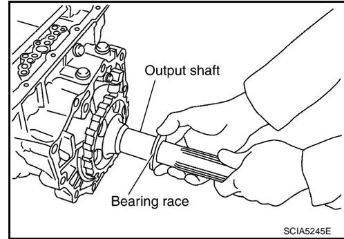
45. Remove output shaft from transmission case by rotating left and right.
