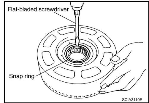
3. Check operation of 3rd one-way clutch.
