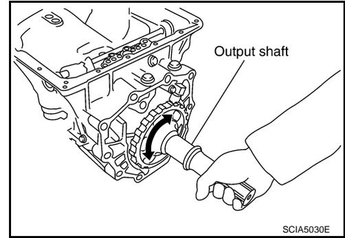
33. Install bearing race to output shaft.
