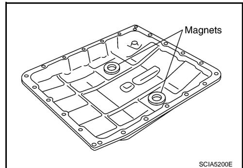
17. Install oil pan to transmission case. Refer to [TM-206, "Oil Pan"](#).
