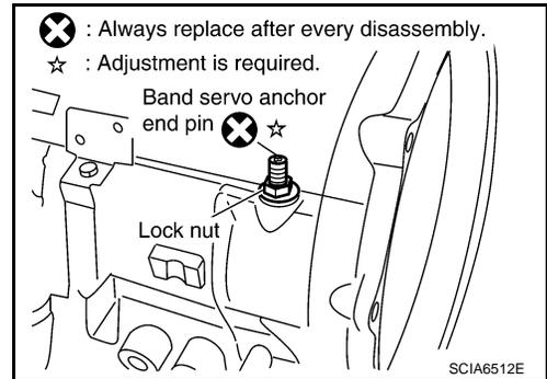
49. Install brake band in transmission case.
