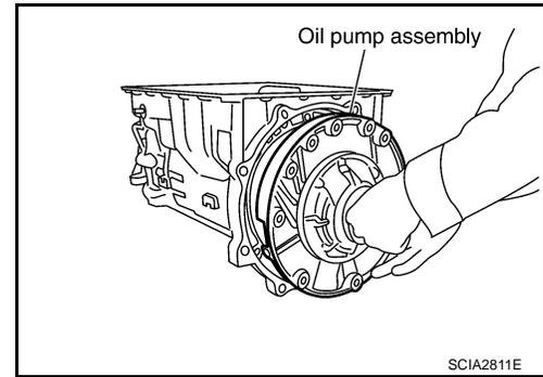
4. Apply recommended sealant (Genuine RTV Silicone Sealant or equivalent. Refer to [GI-15, "Recommended Chemical Products and Sealants"](#).) to oil pump assembly as shown.
