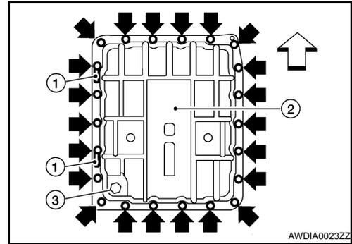
3. Install oil pan bolts and clips tighten in numerical order as shown.
