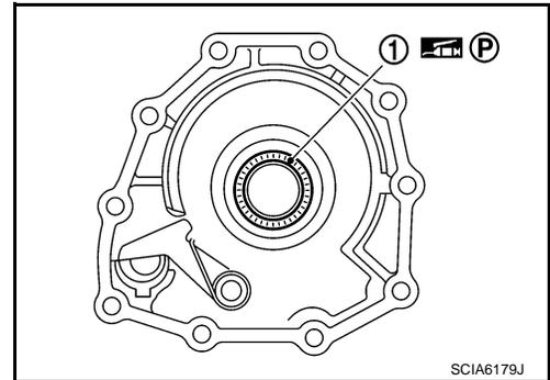
30. Install seal rings to output shaft.
