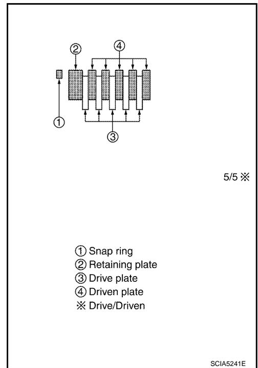
2. Install snap ring in high and low reverse clutch drum using suitable tool.
