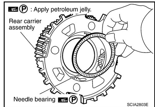
41. Install bearing race in rear carrier assembly.
