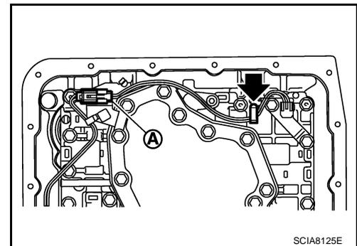
5. Remove A/T fluid temperature sensor 2 with bracket from control valve with TCM.
