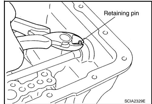
62. Remove manual plate (with parking rod) from manual shaft.
