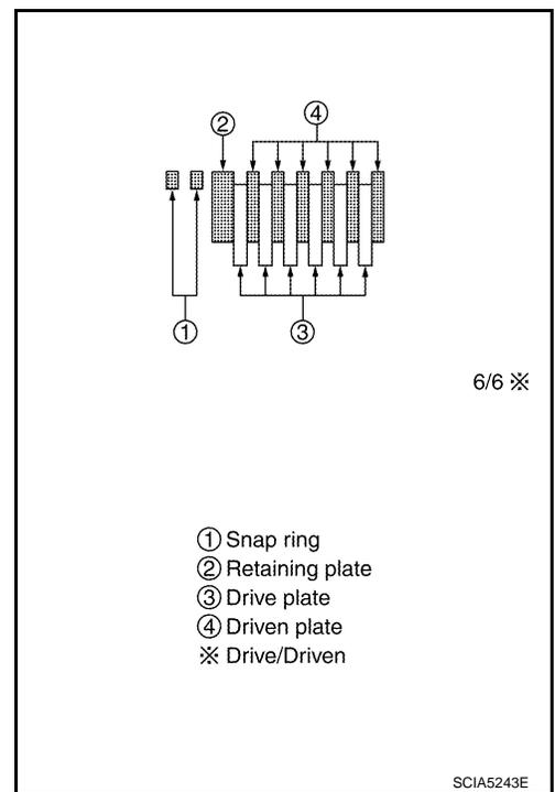
2. Install snap rings in direct clutch drum using suitable tool.
