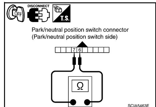
3. If NG, replace the control valve with TCM. Refer to [TM-208, "Control Valve with TCM and A/T Fluid Temperature Sensor 2"](#)
