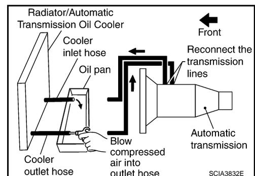
9. Blow compressed air regulated to 5 - 9 kg/cm<sup>2</sup> (70 - 130 psi) through the cooler outlet hose for 10 seconds to force out any remaining fluid.
