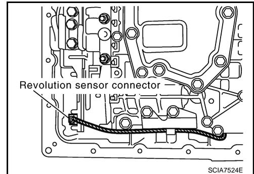
14. Securely fasten revolution sensor harness with terminal clip.
