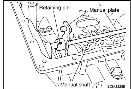
61. Remove manual shaft retaining pin using suitable tool.
