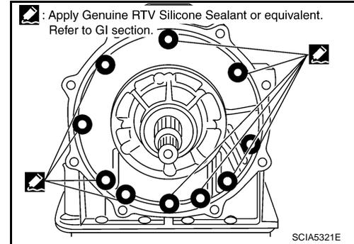
5. Tighten oil pump bolts to specified torque.
