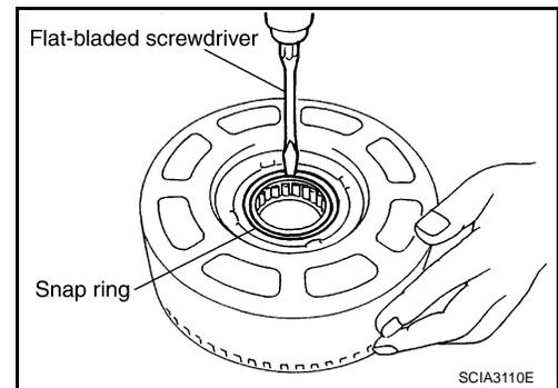
2. Remove 3rd one-way clutch from front sun gear.
