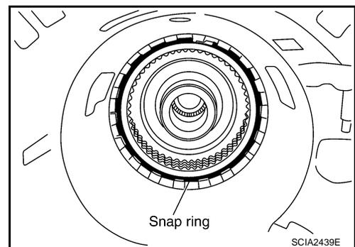
22. Measure clearance (A) between retaining plate and snap ring. If not within specified clearance, select proper retaining plate.
