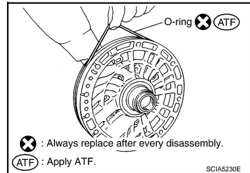
2. Install new O-ring to oil pump housing.
