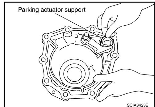
73. Remove parking pawl (with return spring) and pawl shaft from rear extension (2WD models) or adapter case (4WD models).
