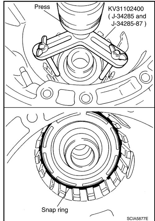
18. Install reversr brake drive plates driven plates and dish plates in transmission case.
