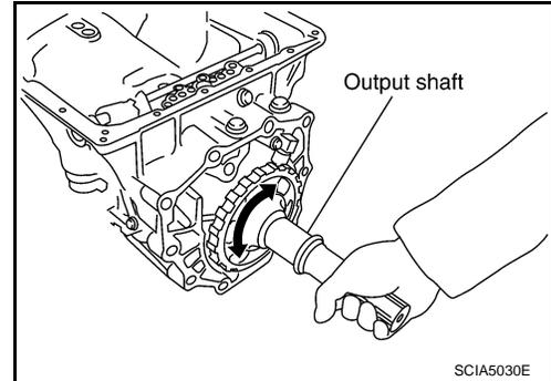
46. Remove parking gear from output shaft.
