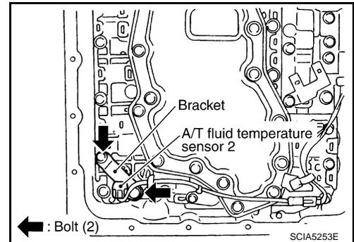
3. Connect A/T fluid temperature sensor 2 connector (A).
