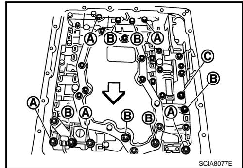
i. Tighten bolt (A), (B) and (C) temporarily to prevent dislocation. After that tighten them in order (A → B → C), and then tighten other bolts.
