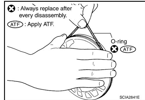
4. Remove O-ring from oil pump cover.
