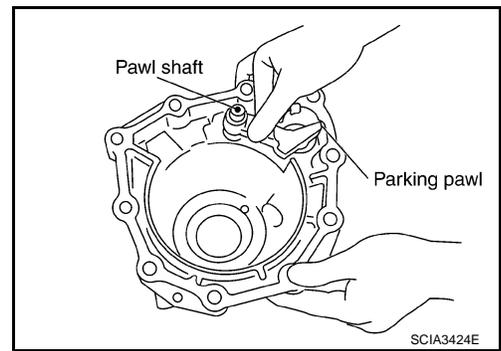
28. Install parking actuator support to rear extension (2WD models) or adapter case (4WD models).
