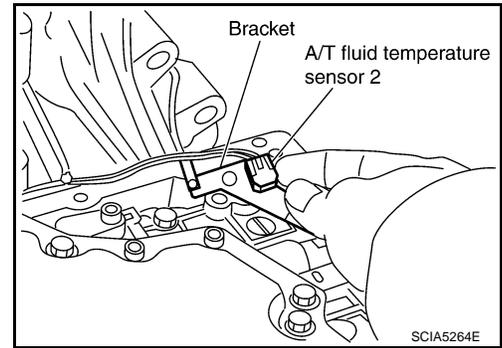
2. Install A/T fluid temperature sensor 2 (with bracket) in control valve with TCM. Tighten A/T fluid temperature sensor 2 bolt to the specified torque. Refer to [TM-224, "Component"](#).
