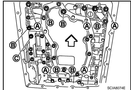
9. Tighten bolt (1), (2) and (3) temporarily to prevent dislocation. After that tighten them in order (1 → 2 → 3). Then tighten other bolts.
