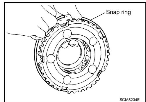
4. Disassemble input clutch assembly.
