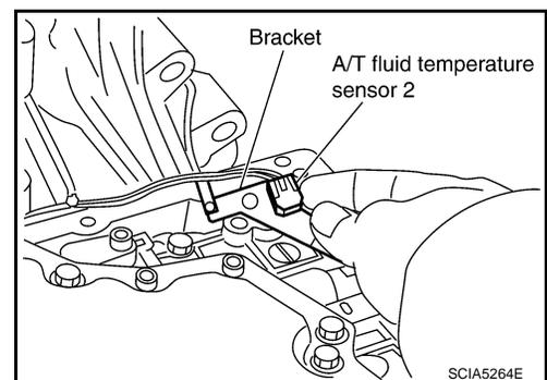
6. Install A/T fluid temperature sensor 2 (with bracket) to control valve with TCM. Tighten A/T fluid temperature sensor 2 bolt to the specified torque. Refer to [TM-224, "Component"](#).
