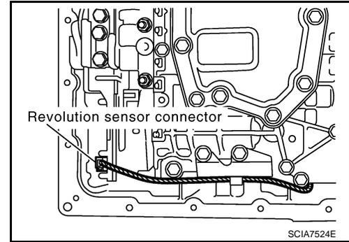
34. Straighten terminal clip to free revolution sensor harness.
