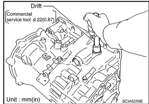
2. Install detent spring and spacer in transmission case and secure with the bolt.
