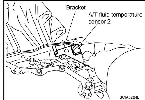
f. Install A/T fluid temperature sensor 2 (with bracket) to control valve with TCM and tighten bolt to specified torque.
