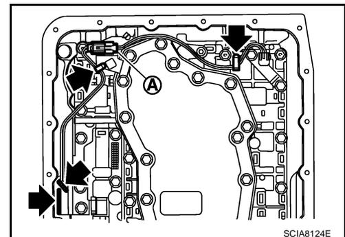
9. Straighten terminal clip to free the revolution sensor harness.
