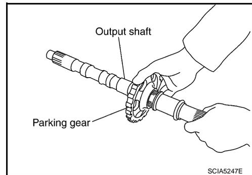
47. Remove seal rings from output shaft.
