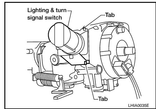
5. Remove the screws, release the clip, and remove the spiral cable.
