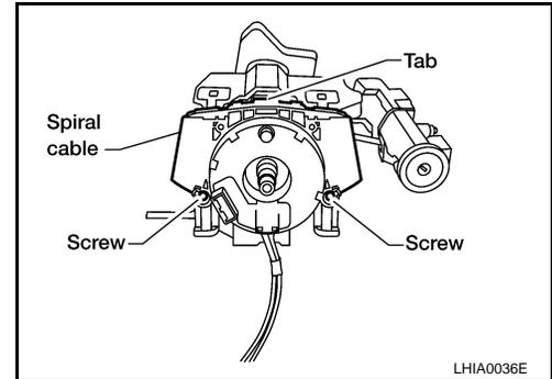
6. Remove the spiral cable connectors.
