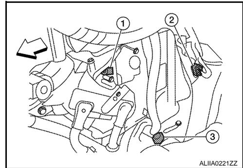
11. Disconnect the ducts from the rear heater and cooling unit assembly. Refer to [VTL-33, "Component"](#).
