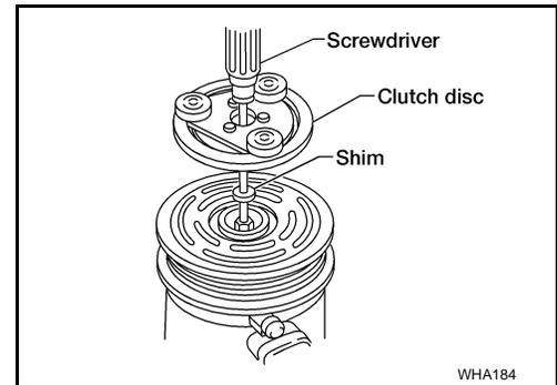
5. Install the clutch pulley bolt using Tool, to prevent the clutch disc from turning and tighten the bolt to specification.
