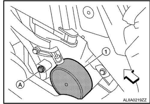
9. Remove the rear high- and low-pressure pipes bolt (A) to disconnect the rear high- and low-pressure pipes from the rear expansion valve (1).
