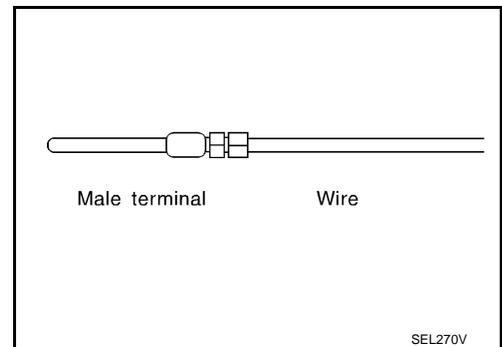
3. While holding the wire of the male terminal, try to insert the male terminal into the female terminal.
