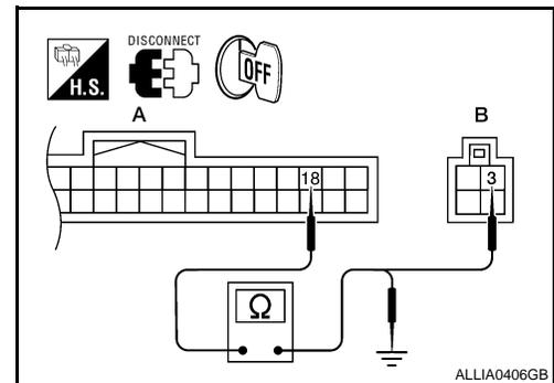
4. Check continuity between BCM harness connector M18 (A) terminal 18 and ground.
