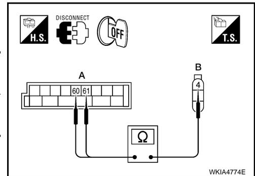
5. Check continuity between the BCM harness connector M20 and the door mirror connectors (if equipped with turn signals in the mirrors).
