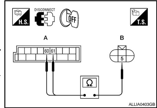
4. Check continuity between the BCM harness connector M20 and the rear combination lamp connectors.
