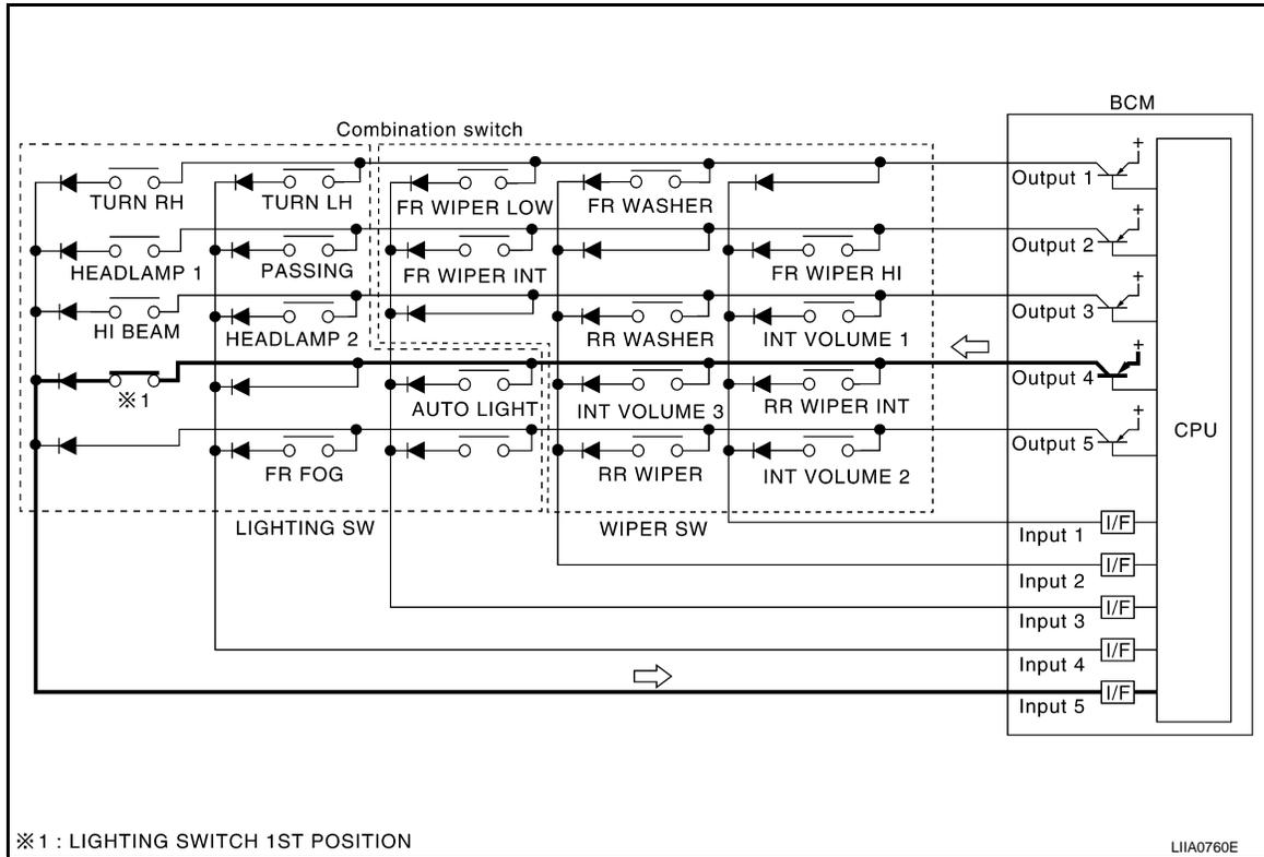
Combination switch INPUT-OUTPUT system list
