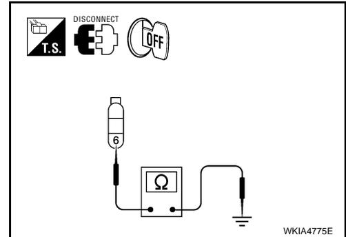
3. Check continuity between the door mirrors and ground (if equipped with turn signals in the mirrors).
