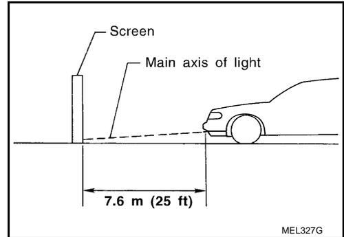
3. Adjust front fog lamps using adjusting screw so that the top edge of the high intensity zone is 100 mm (4 in) below the height of the fog lamp centers as shown.
