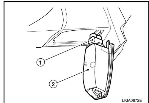
4. Pull to remove puddle lamp bulb (2) from puddle lamp socket (1).
