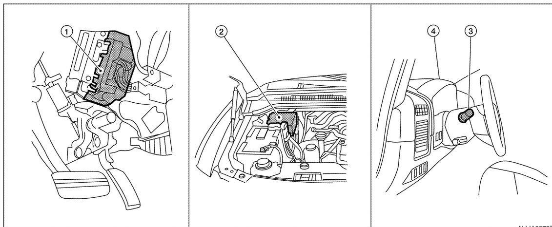
1. BCM M18, M20 (view with instrument panel removed)
