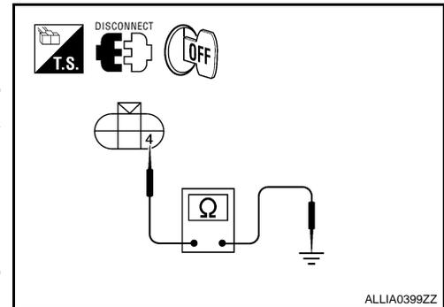
2. Check continuity between the rear combination lamp harness connectors B70 and B130 terminal 3 and ground.
