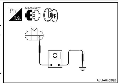
2. Check continuity between the rear combination lamp harness connectors and ground.
