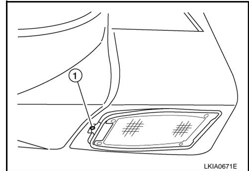
2. Lower outer edge and slide puddle lamp housing out of door mirror.
