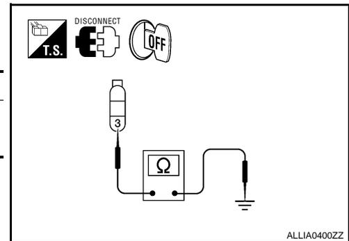
3. Check continuity between the license plate lamp harness connectors and ground.
