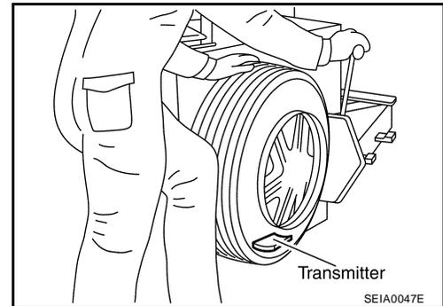
3. Turn tire so that valve hole is at bottom, and gently bounce the tire to ensure transmitter is near valve hole. Carefully lift tire onto turntable and position valve hole (and transmitter) 270 degrees from mounting/dismounting head.
