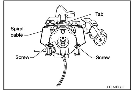
6. Remove the spiral cable connectors.
