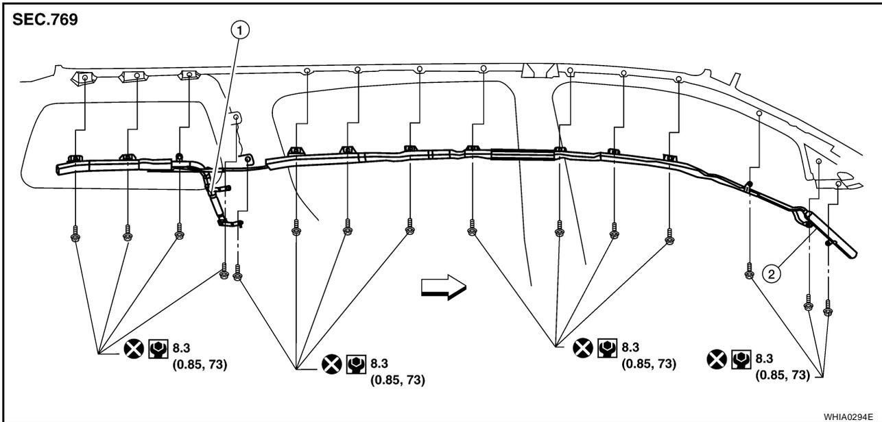
1. Rear side curtain air bag module connector      2. Front side curtain air bag module connector      ← Vehicle front connector
