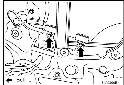
6. Remove the bolts, and the regulator and guide channel.
