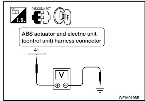
**4. STOP LAMP RELAY CIRCUIT INSPECTION**
