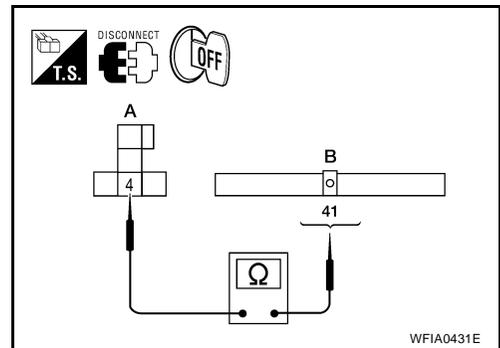
**ABS/TCS/VDC Control Unit Power and Ground Systems Inspection**
