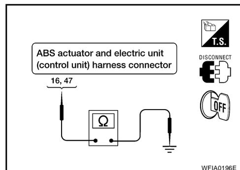
**ABS Warning Lamp Stays On When Ignition Switch Is Turned On**
