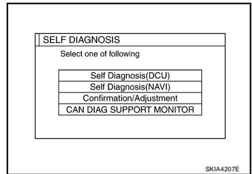
5. When "Confirmation/Adjustment" is selected on the initial self-diagnosis screen, the operation will enter the CONFIRMATION/ADJUSTMENT mode. In this mode, check and adjustment of each item will become possible.
