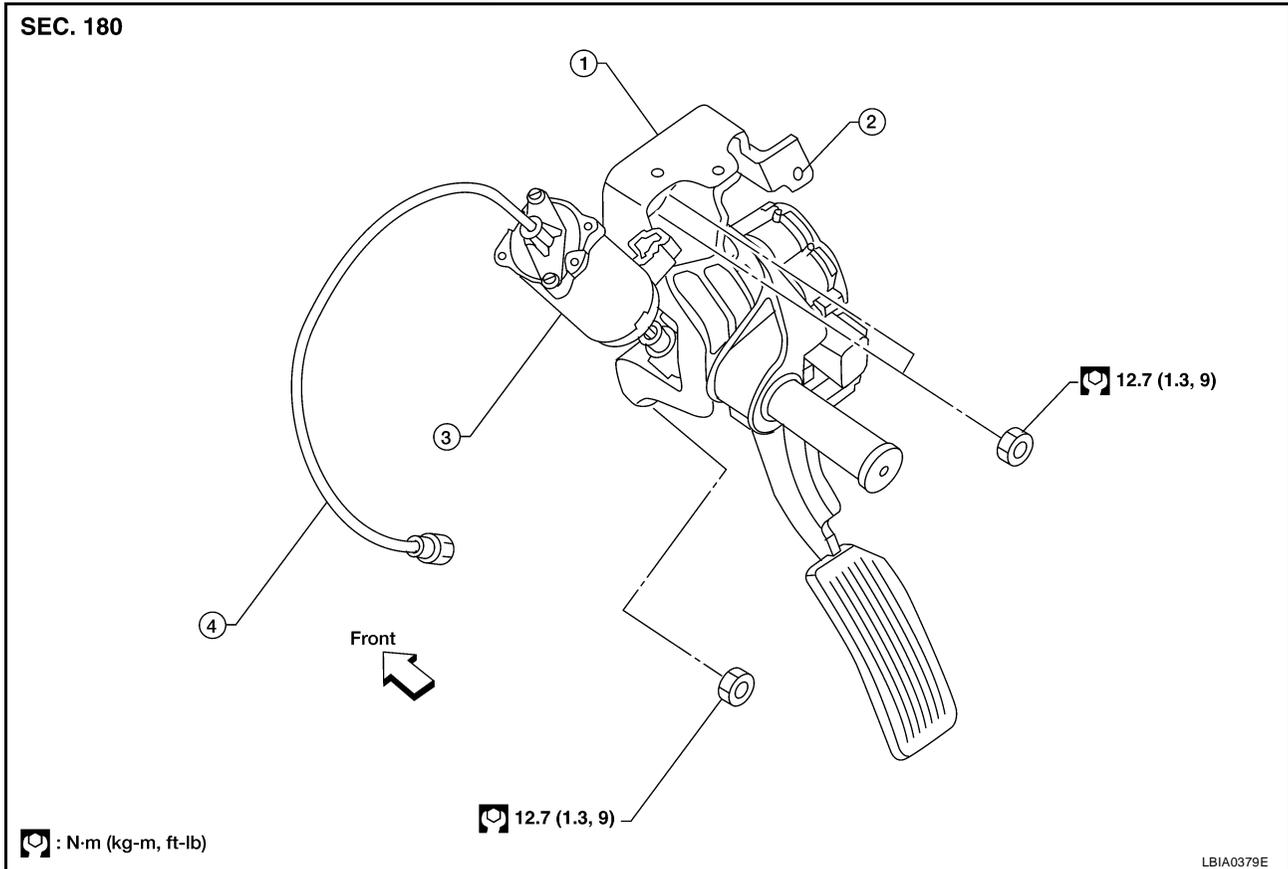
1. Adjustable accelerator pedal assembly
